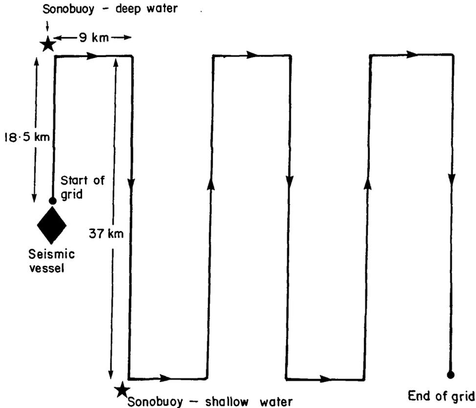
FIG. 2. Grid pattern used to survey areas near geophysical vessels.
